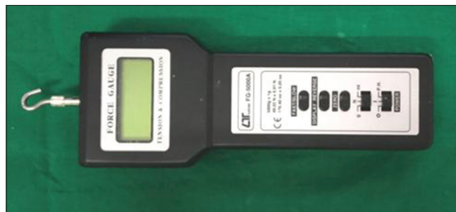
Figure 5: Digital force gauge with the hook (FG 5000A, Lutron Electronic Enterprise Co., Ltd. Taipei)
